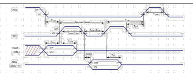
Table 17.3.2.1: 3-pin Serial Interface Characteristics
