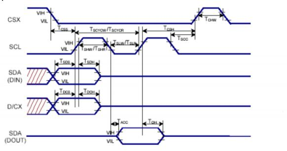
Table 17.3.2.2: 4 pin Serial Interface Characteristics
