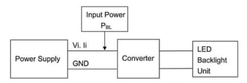
Note 3: The "LED life time" is defined as the module brightness decrease to 50% original brightness at Ta=25°C and If =30mA. The LED lifetime could be decreased if operating If is larger than 30mA. Note 4: LED light bar circuit:
