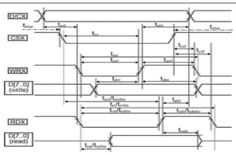
Note: Logic high and low levels are specified as 30% and 70% of VDDI for Input signals.
